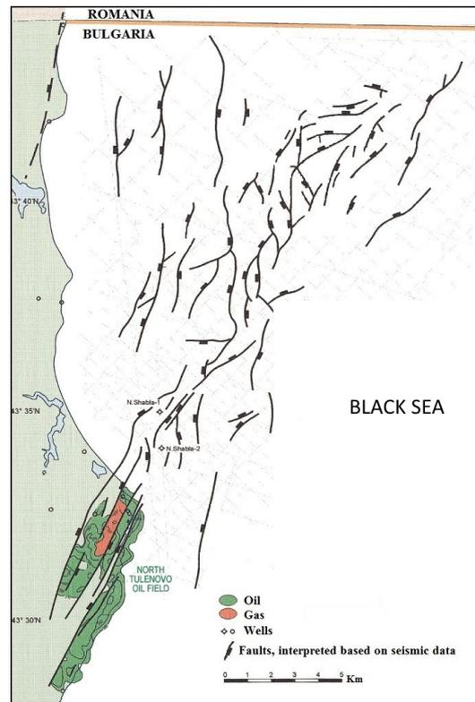
Fig. 11 – The NE-SW fault system, shown on strike with the Tyulenovo structural trend, and the N-S fault system, both depicted at top Valanginian carbonate based on reflexion seismic data interpretation (modified after Bottomley & Pritchard, 1998).
