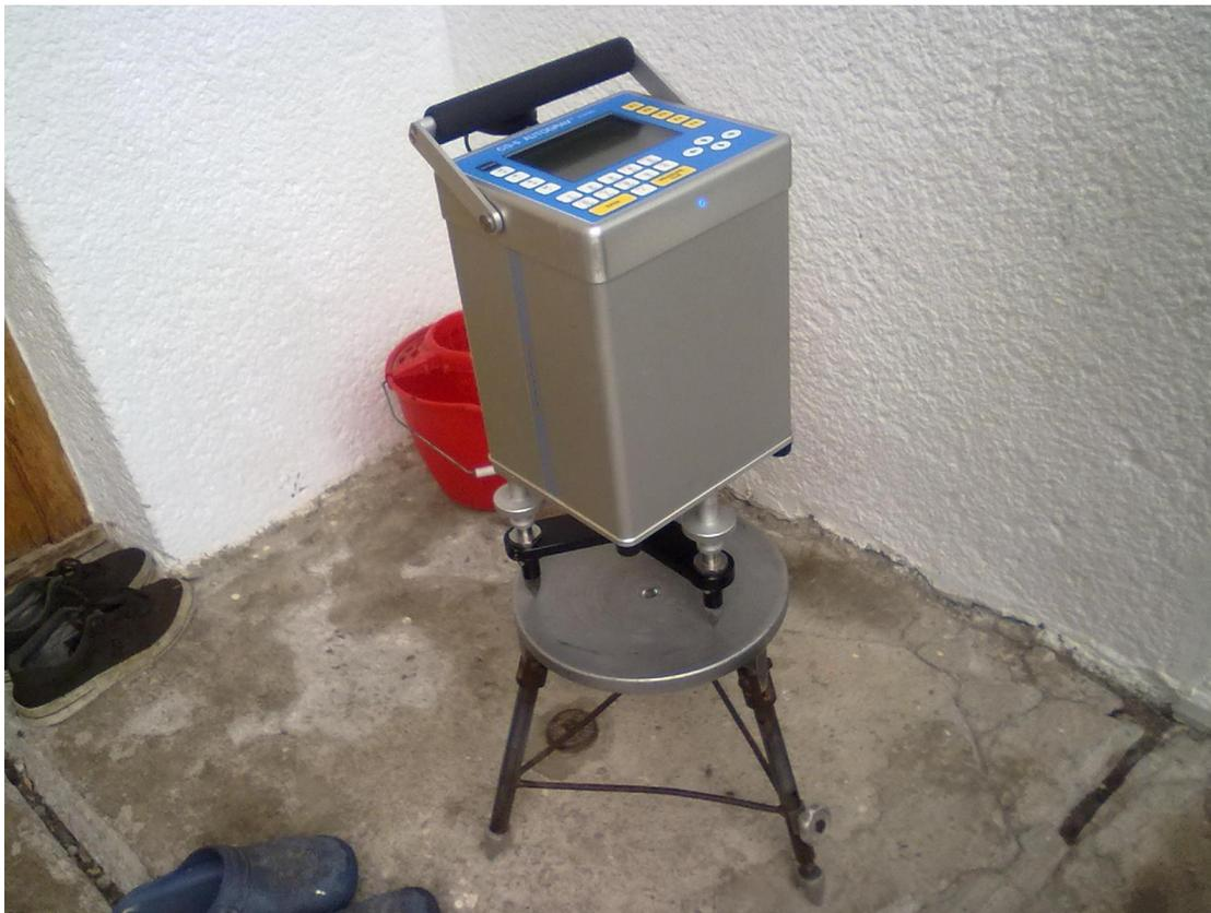
**Fig. 30 - CG-5 AUTOGRAV METER OPERATED IN THE CENTRAL BASE-STATION OF THE 2014 SURVEY: LEPSA FROM THE 2<sup>nd</sup> ORDER GRAVITY NETWORK OF ROMANIA**
