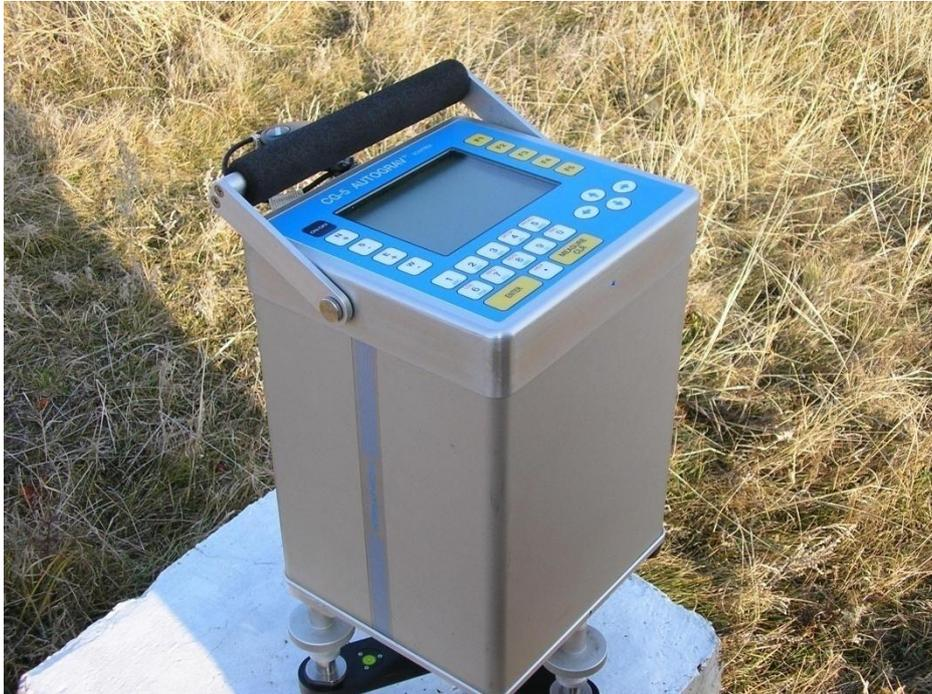
**Fig.18 - Scintrex CG-5 AUTOGRAV gravity meter**
