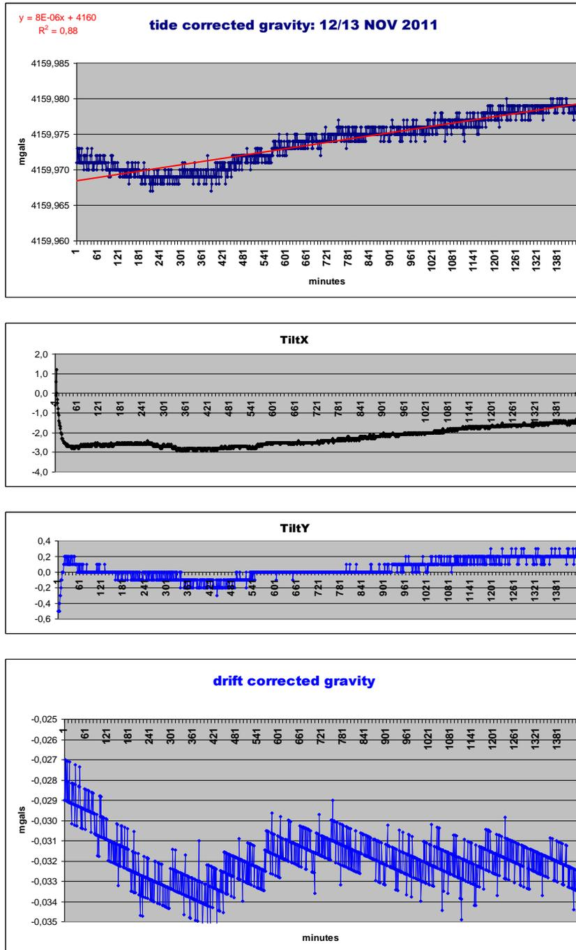
**Fig. 20 - Improving the reading reproducibility of Scintrex CG-5 gravity meter by introducing the additional drift correction. Tilt X-inclination along  $O_x$ , Tilt Y – inclination along  $O_y$ . Tests conducted in DDGT gravity lab.**
