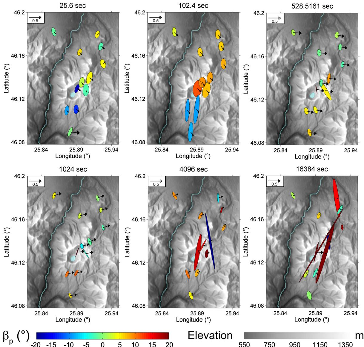
Fig. 7. The phase tensor ellipses and real induction arrows (in the so-called Wiese convection) in the horizontal map at six periods. The fill of ellipses represents the  $\beta_p$  skew angle in degree (Wiese, 1962; Caldwell et al., 2004).
