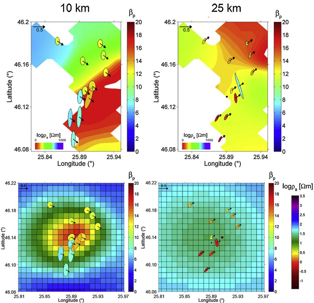
**Fig. 10.** Comparison of 2-D and 3-D inversion results, shown in the form of maps at apparent depths of 10 and 25 km. The fill of ellipses represents the  $\beta_p$  skew angle in degree. Resistivity values are in logarithmic scale.
