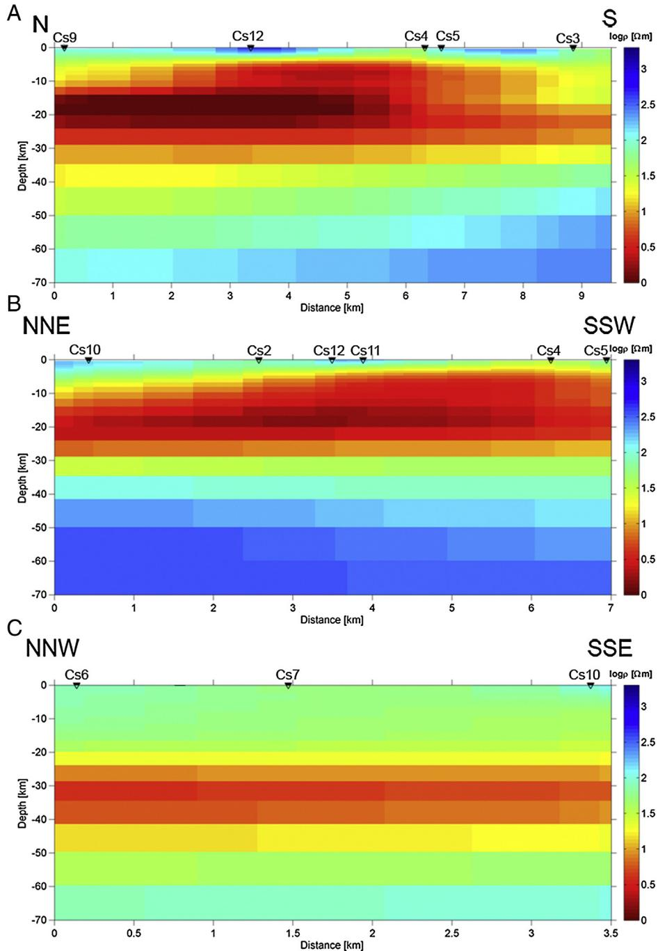
**Fig. 8.** 2-D inversion results along three selected profiles. Bimodal inversion with  $H_z$  conjugate was applied, based on inversion code by Rodi and Mackie (2001). Resistivity values are in logarithmic scale: a) NS profile with sites: 9-12-4-5-3 (RMS 5.6%); b) NNE-SSW profile with sites: 10-2-12-11-4-5 (RMS 2.075%); c) profile 6-7-10 (RMS 0.88%).
