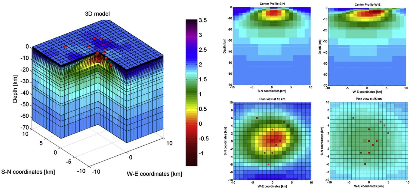
**Fig. 9.** 3-D model of the investigated area by 3-D inversion results in different view. Resistivity values are in logarithmic scale. The MT stations are shown by red dots. (For interpretation of the references to color in this figure legend, the reader is referred to the web version of this article.)
