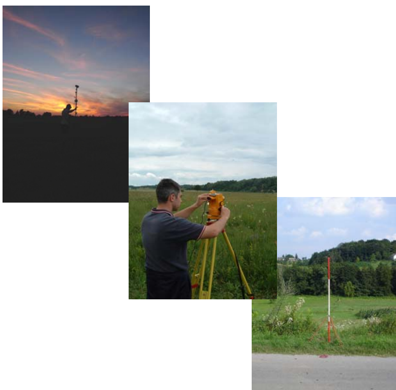
Fig. 1: Gradiometry (left). Besides investigating the condition of low total intensity gradients in repeat station setup, gradiometry is important in site maintenance as an indication of possible site's contamination. Orientation of the theodolite in reference to the azimuth reference mark (middle). The azimuth reference mark with a signal rod (right) was usually placed near the road, within the distance of a few hundred meters.
