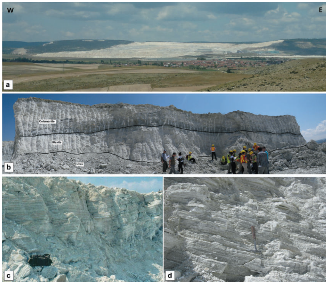
Figure 5. (a) Kırka Sarıkaya opencast borax mine, Eskişehir county; (b) View of Sarıkaya quarry with ulexite layers alternating with nodular and massive lithofacies of colemanite. Crystalline masses, vugs, geodes, and veins can be observed, in the upper section of the Sarıkaya opencast deposit; (c) Alternating borax layers and dolomitic clays; (d) Laminated lithofacies of borax (brown material) alternating with dolomitic, marly laminae (white laminae). Laminated borax lithofacies with palisade fabric in borax laminae. Clear material corresponds to lutitic matrix and laminae (dolomitic claystone). Dark material corresponds to fresh, crystalline borax.
