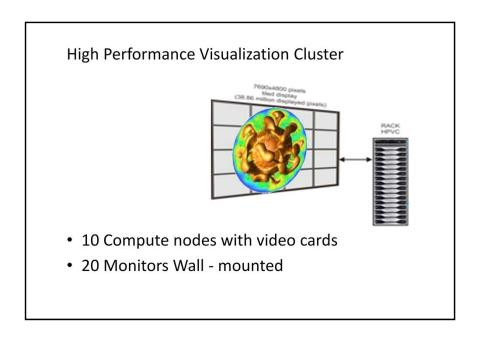
The visualization cluster is designed to be a subset of the "main" computing cluster. As such, a third of the nodes have video cards capable to operate two monitors. The models seen by their authors on this wall of monitors will be examined in greater detail, and this will help improve them.
