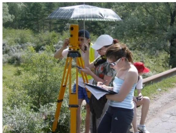
Figure 3.2.2. Students of the Faculty of Geodesy performing geometric levelling works within the geodynamic micro-polygon no. 1.
