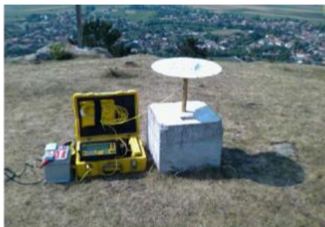
Fig. 3.2.7. GPS observations conducted on the P115 Sânzieni benchmark.
