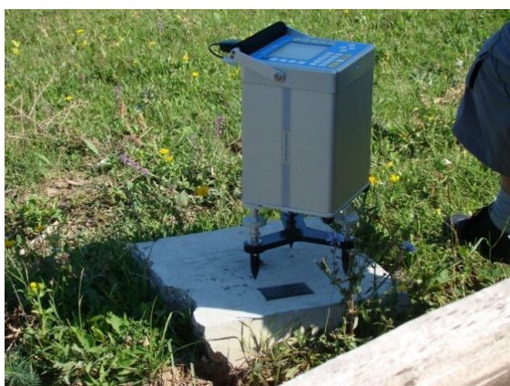
Figure 2.7. Scintrex CG5 AUTOGRAV #40387 gravity meter operated on a gravity benchmark within the Tulnici–Valea Sării–Vrâncioaia micro-polygon.
