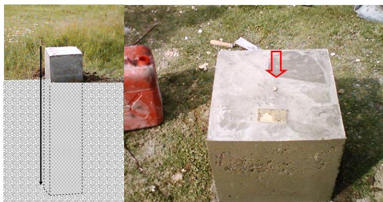
Figure 2.6. The Romanian geodynamic network benchmarks. The arrow marks the device for centring the GPS antenna.
