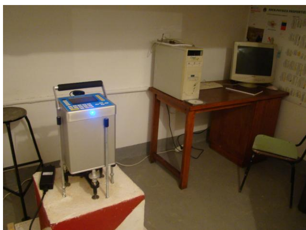
Fig. 2.1. Scintrex CG5 gravimeter #40387 operated on the pillar of the gravity laboratory.
