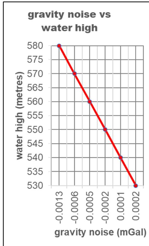
Figure 7 – Potential gravimetric noise induced by various levels of water in the Nehoiășu hydropower plant reservoir at the location of the Siriu VDBG base station.
