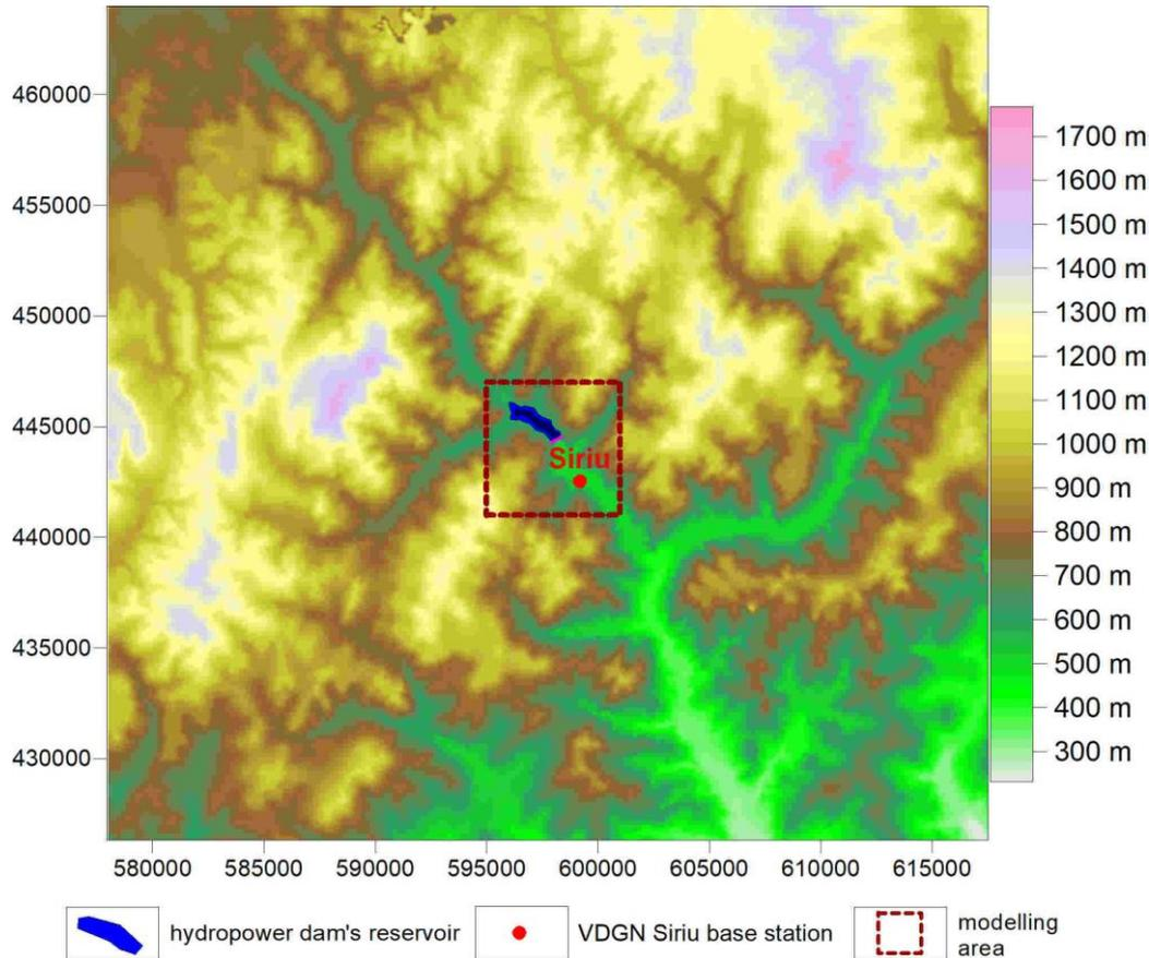
Figure 3 – Digital terrain model of the Siriu hydropower dam area and location of the gravity station.
