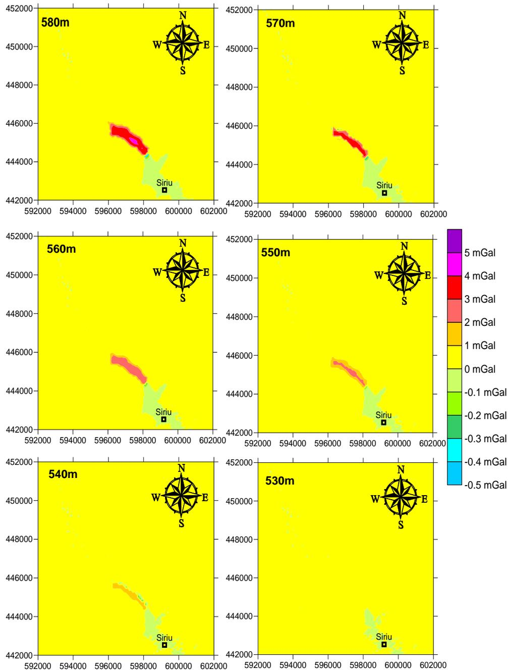
Figure 6 – Gravity noise for various water levels in the Siriu hydropower plant reservoir.
