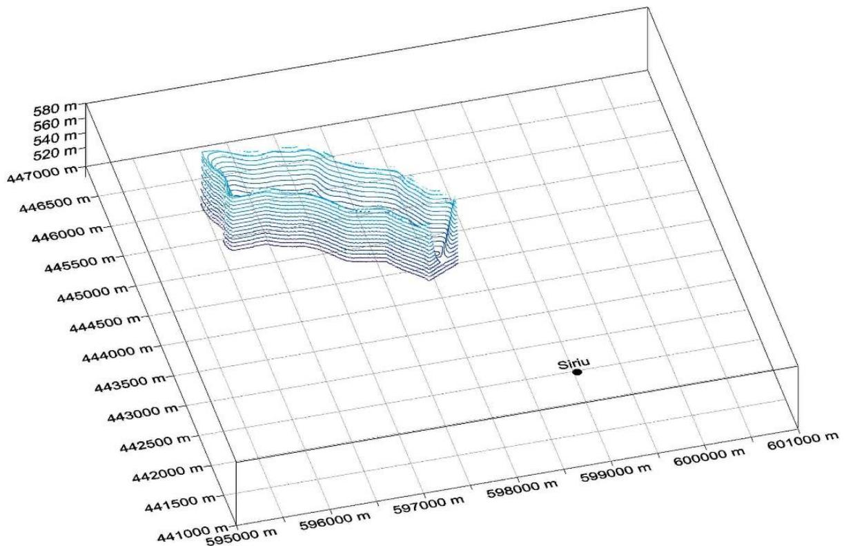
Figure 5 – 3D geometry of the water bodies considered for the simulation of the gravity effect.
