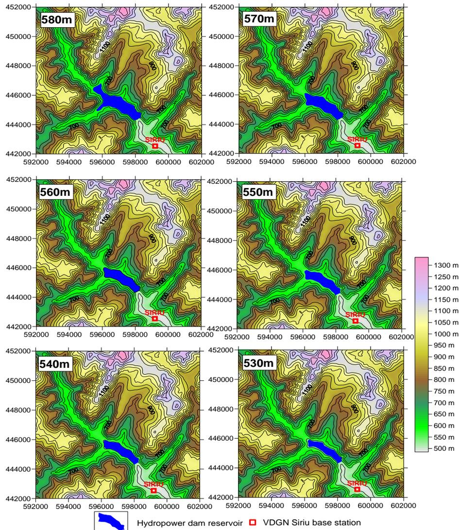
Figure 4 – Digital models including topography and water surface serving as inputs in the simulation of gravity effect of the water level at the Siriu hydropower dam (the altitude of the water level is mentioned in the upper left corner of each map).
