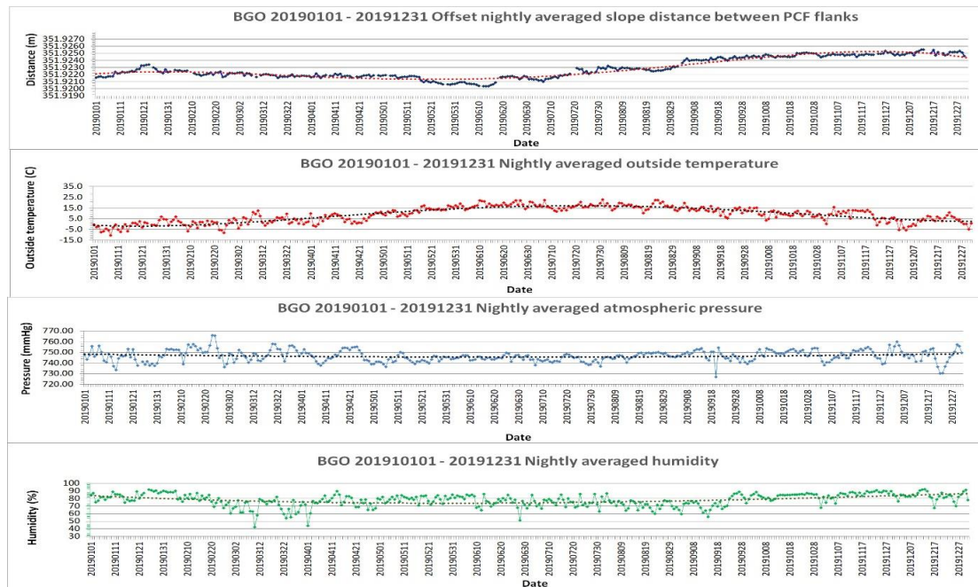
Figure 10 – 2019 Offset nightly averaged slope distance between PCF flanks versus nightly averaged atmospheric parameters.
