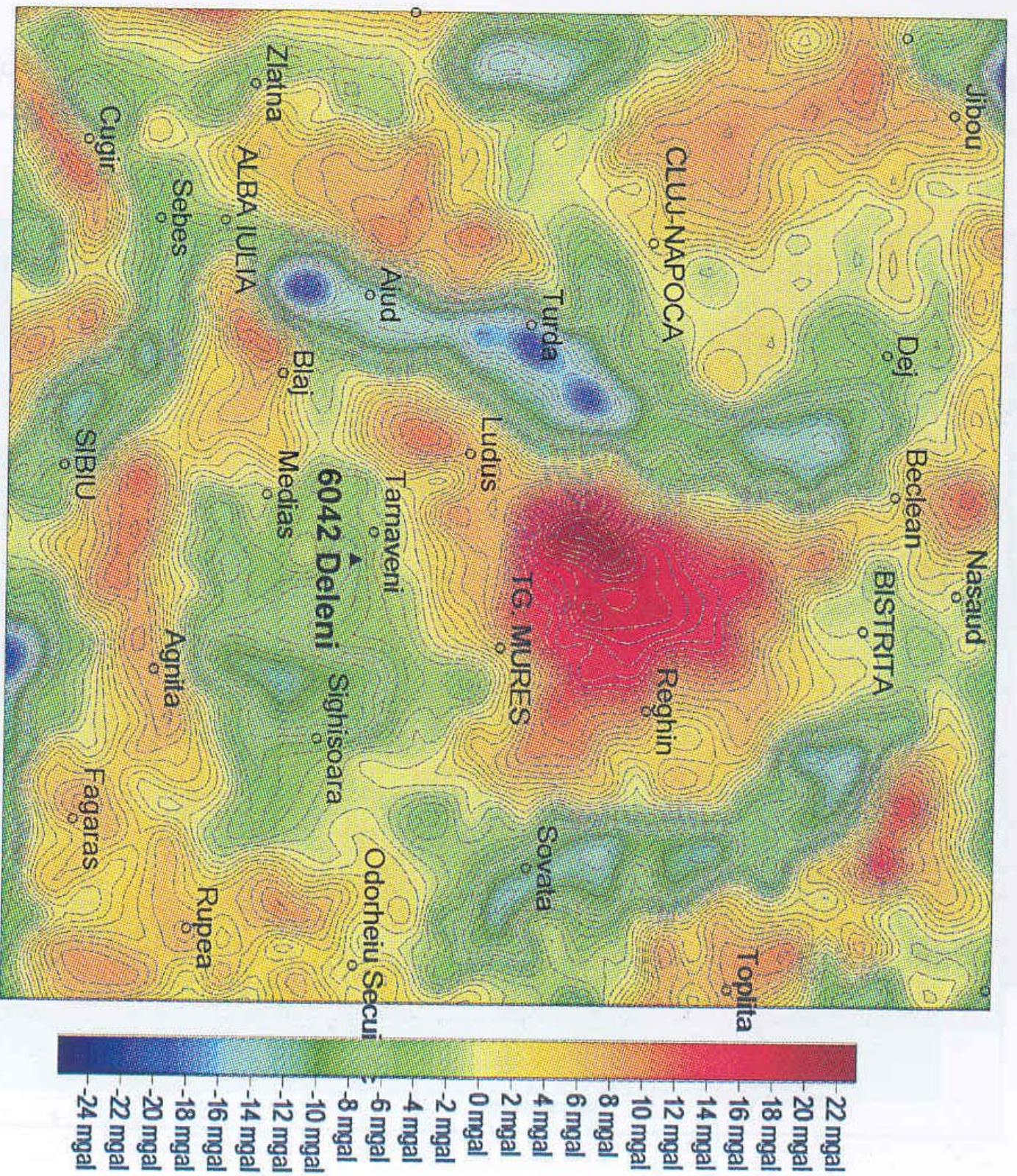
Fig. 3 – Residual gravity anomaly within the 6042 Deleni well region. A 5th order polynomial trend has been removed from data.
