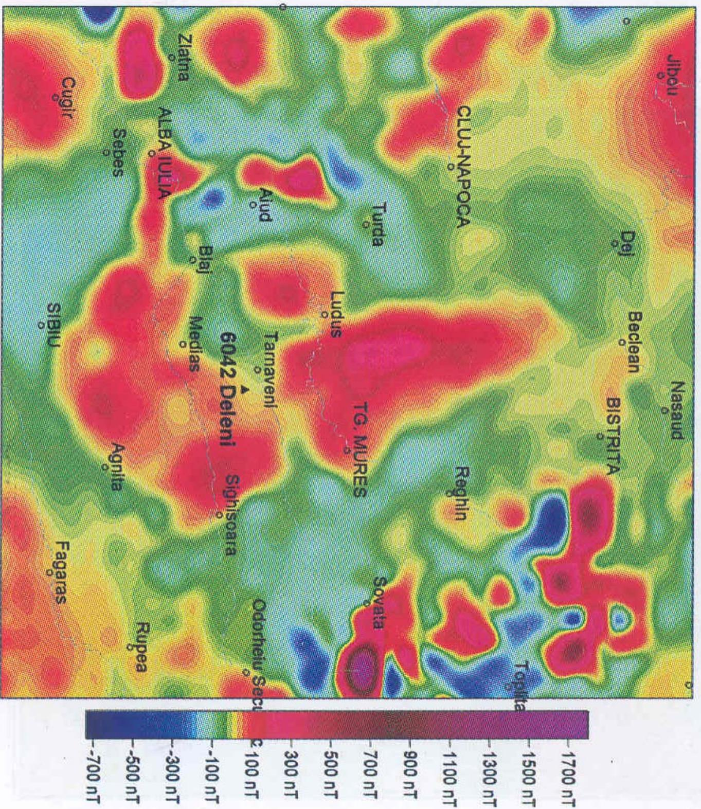
Fig. 5 – Residual ground vertical component geomagnetic anomaly within the 6042 Deleni well region. A 5th order polynomial trend has been subtracted from data (raw data according to Airinei *et al.*, 1983).
