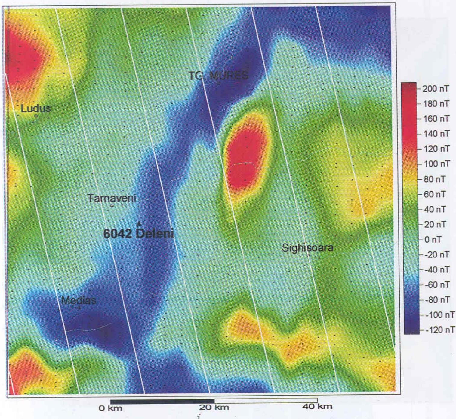
Fig. 6 – Reflection of the deep located geomagnetic zones in the total intensity residual geomagnetic anomaly as obtained after removing a first order polynomial trend from the aeromagnetic anomaly in the study area. White lines mark the geomagnetic reference field trend.
