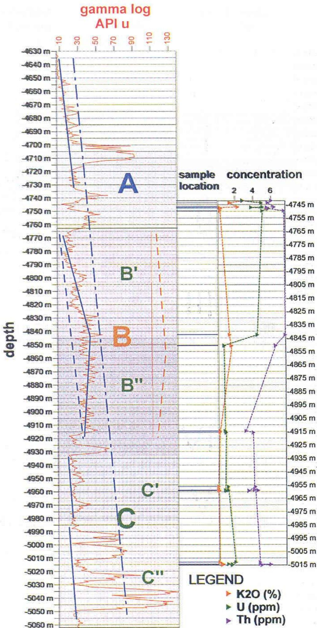
Fig. 8 – Gamma log interpretation and geochemistry of the core samples (geochemistry data according to Hoeck & Ionescu, 2003).
