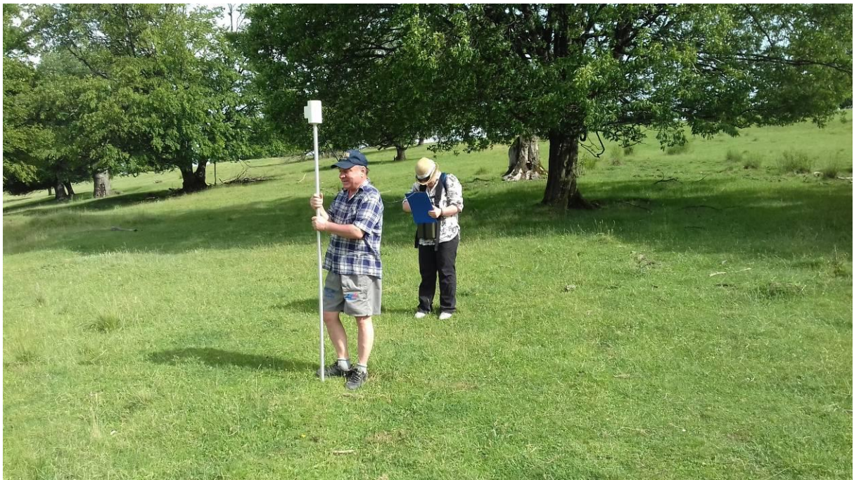
Fig. 4.2.2.3.1 Geometrics G856 AX run along an observational line
