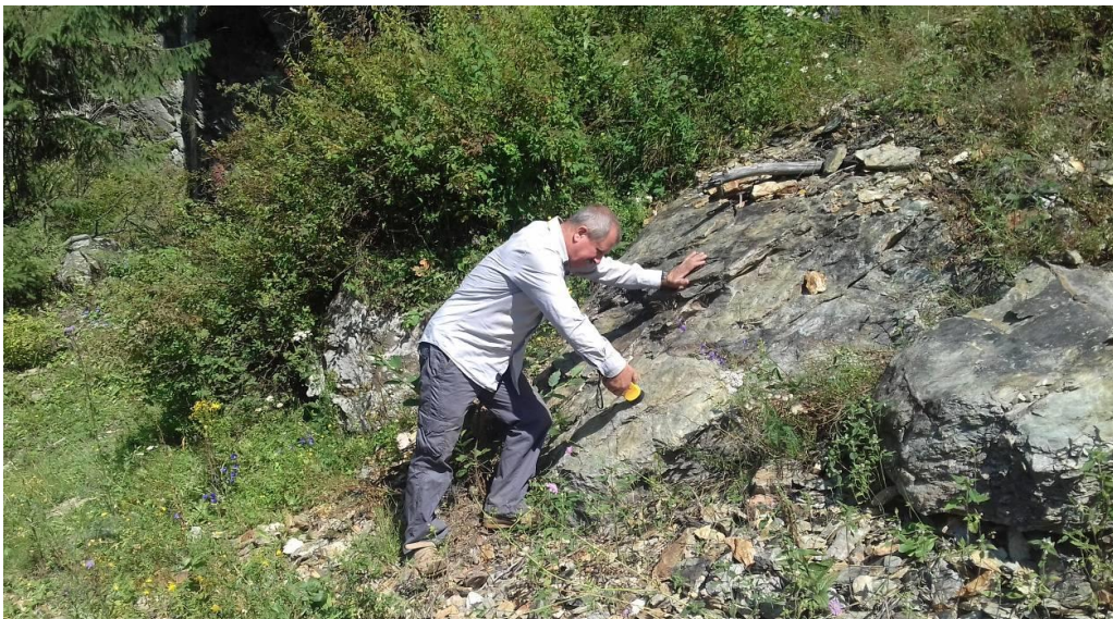
Fig. 4.2.2.4.2 Dr. Mykhailo Orlyuk with the Instiute of Geophysics, National Academy of Sciences of Ukraine, probing magnetic susceptibility on an outcrop
