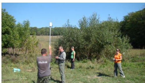
Fig. 2 Magnetic survey jointly conducted by Romanian and Ukrainian specialists within Baspunaru area
