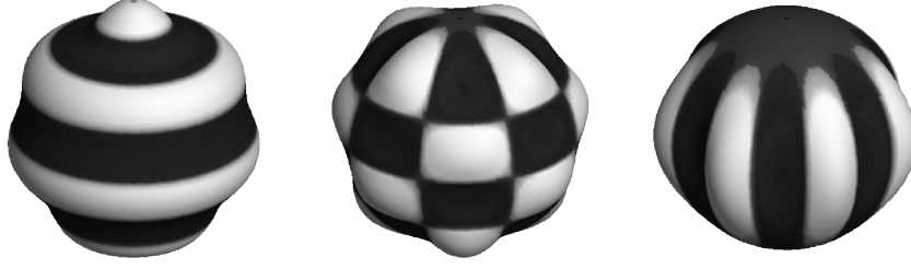
Figure 3: Zonal harmonics, for n = 7 and m = 0 (left), tesseral harmonics, for n = 7 and m = 4 (middle), and sectorial harmonics, for n = 7 and m = 7 (right). Figures provided by prof. M.Mandea.
