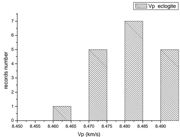
Fig. 5 – Histogram of P-wave propagation velocities determined in the laboratory for eclogite.
