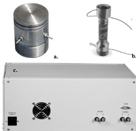
Fig. 3 – The device for elastic wave velocity measurement using ultrasound. a) planar sensor for measuring of velocities P and S; b) receiver-transmitter group assembled for testing of sediment samples; c) transmitter, receiver and the signal conditioning unit.
