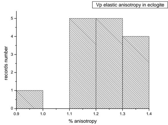
Fig. 7 – Histogram of P wave propagation velocity anisotropy in eclogite determined in the laboratory.
