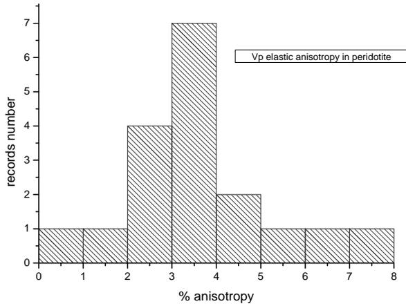
Fig. 6 – Histogram of the elastic anisotropy for the P waves in peridotite determined in laboratory.
