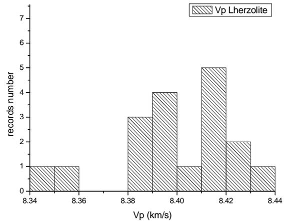
Fig. 4 – Histogram of P-wave propagation velocities determined in the laboratory for lherzolite.
