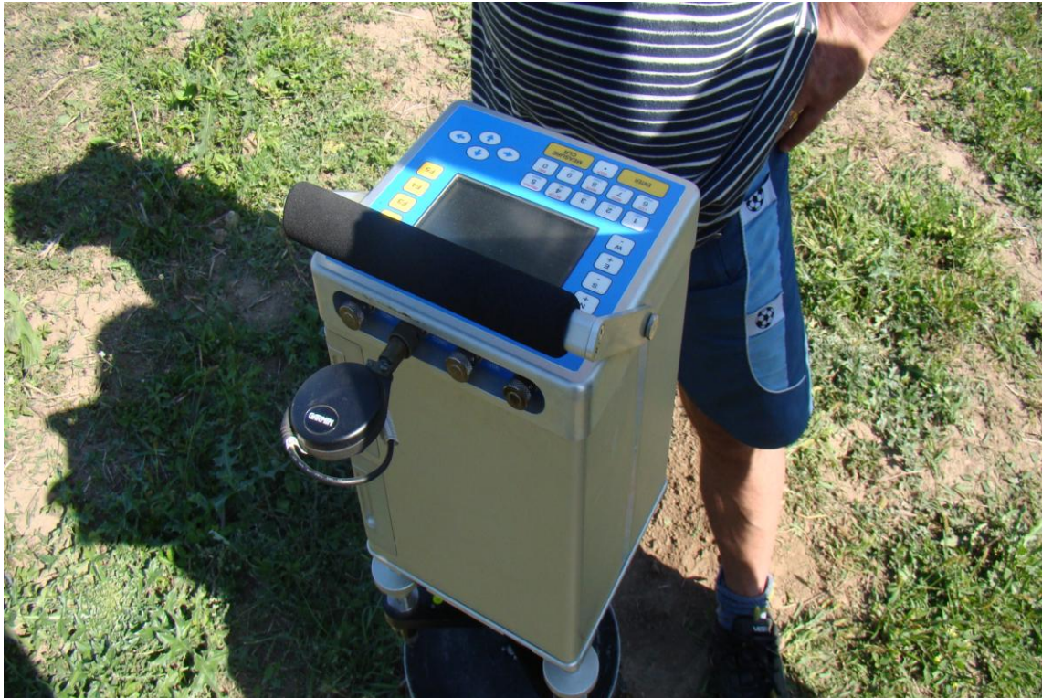
Fig. 31 - CG-5 AUTOGRAV METER OPERATED IN A CURRENT STATION IN THE FIELD
