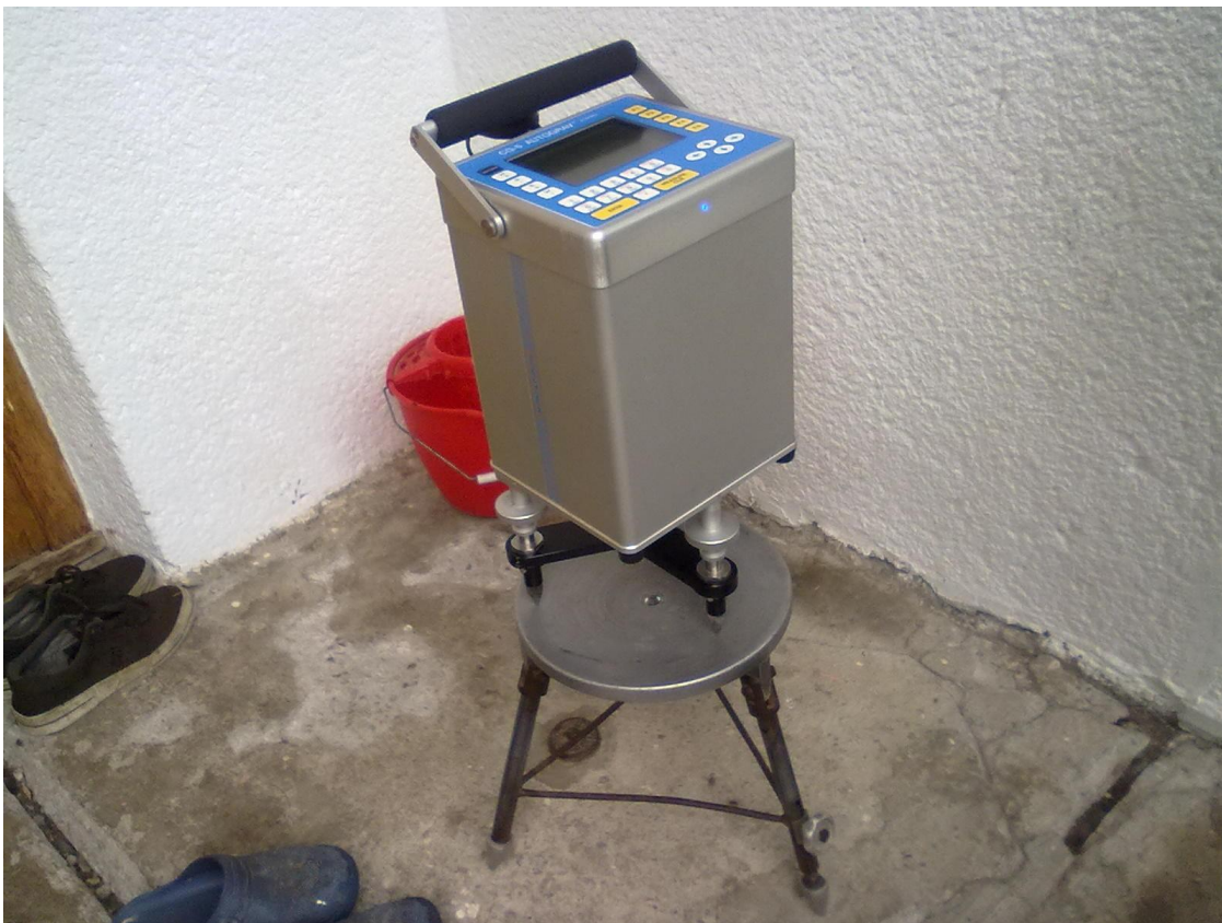
Fig. 30 - CG-5 AUTOGRAV METER OPERATED IN THE CENTRAL BASE-STATION OF THE 2014 SURVEY: LEPSA FROM THE 2nd ORDER GRAVITY NETWORK OF ROMANIA
