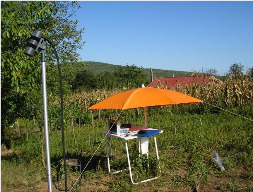
FIG. 33 - SCINTREX SM-5 NAVMAG OPERATED FOR DIURNAL ACTIVITY SERVICE
