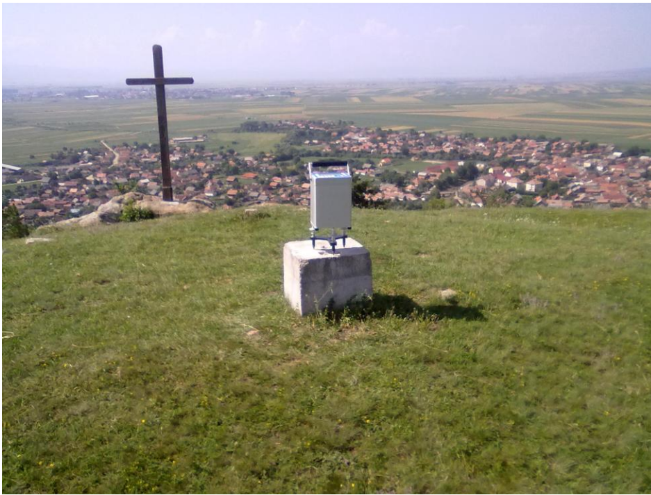
Fig. 29 - CG-5 AUTOGRAV METER OPERATED ON THE P116-SANZIENI (TG. SECUIESC) PILLAR OF THE GRAVITY REFERENCE NETWORK
