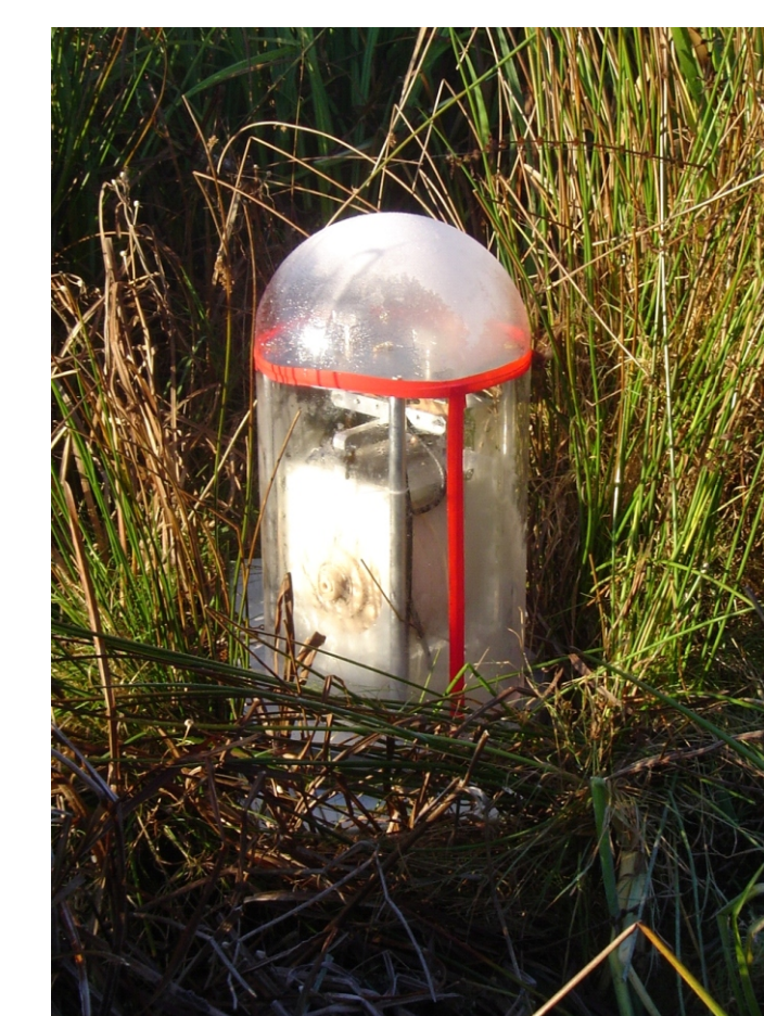
Figure 6. Morning picture of the suspended DIDD magnetometer set up in a muddy area
