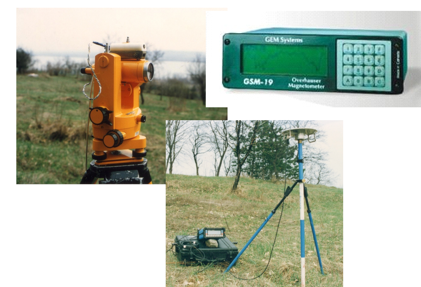
Figure 5. Set of instruments applied for the last repeat station campaigns: DI fluxgate magnetometer installed on Zeiss Theo 020B theodolite for declination, inclination measurements (upper left), GSM-19 Proton Overhauser magnetometer for the total field observations (upper right), and a pair of Ashtech MXII GPS receivers to ensure the accurate bearing in case of missing reference azimuth (down).
