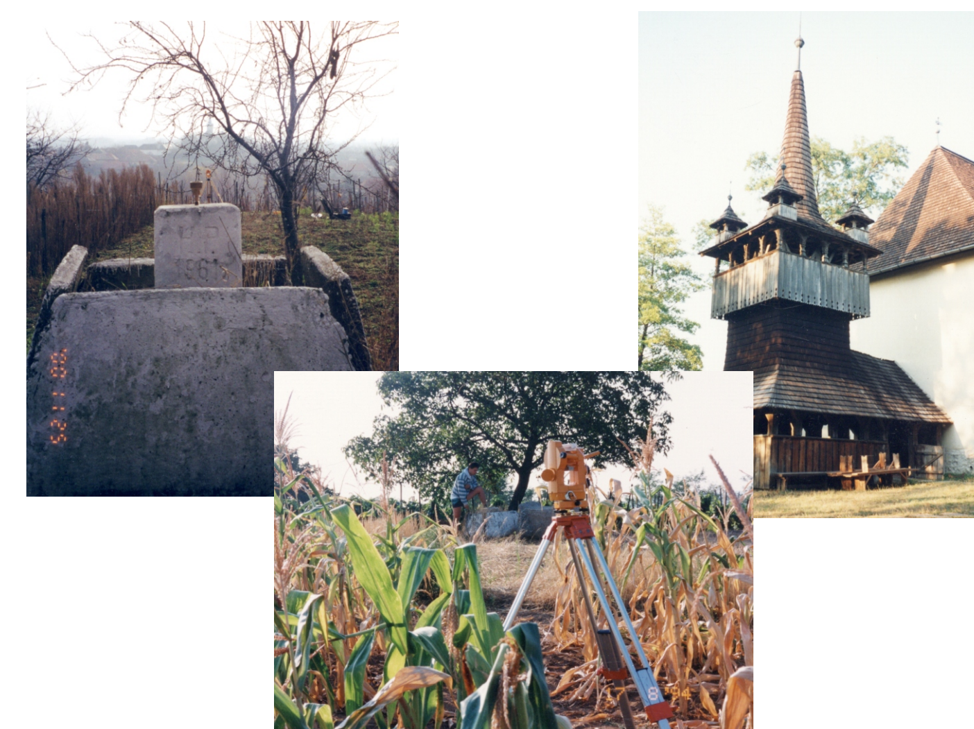
Figure 2. Geodetic reference mark used for the marking of the Hungarian repeat stations (upper left), a tower of church, as a reference azimuth for the declination measurements (upper right), and the DI instrument installed at a distance of about 20 m away from the reference stone (down).
